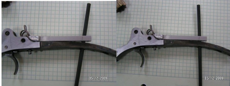
Figure #2 Before and After Elongating main spring screw bore.
