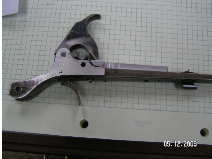
Figure # 7 Properly Assembled SliX-Main System, ready to install
